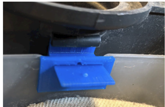
Figure 8: Example of a vacuum cleaner clip 3D-printed during a repair Masterclass of the Sharepair project 1
