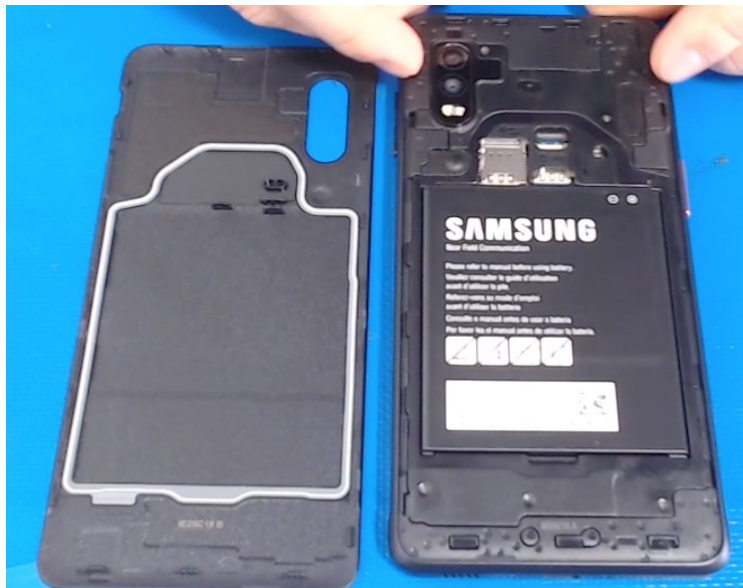
Figure 6: Galaxy XCover Pro back cover with water tight seal
