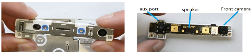
Figure 7: Fair phone module (left) consisting of aux port, speaker, and front camera. Further disassembly of the module shows all these components are permanently attached to a single chip (bottom)
