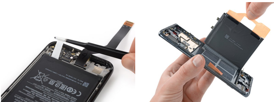
Figure 5: A smartphone battery joined with stretch release adhesive (left) and pull-tab adhesive (right).
